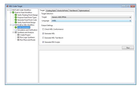
**Tip** You can use the **Target**, **Coding Style**, **Clocks and Ports**, **Test Bench**, and **Optimizations** tabs to set code generation options. For more information, see the HDL Coder Workflow Advisor reference.
