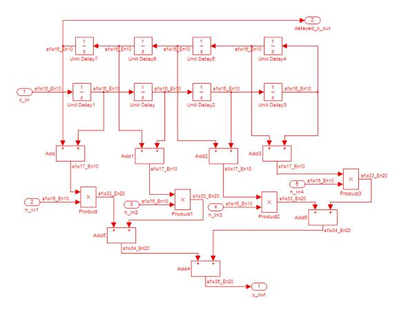
The following figure shows the symmetric\_fir subsystem.
